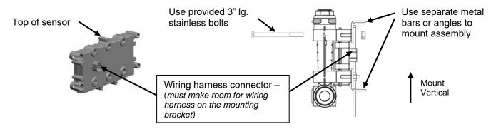
The sensors interlock with each other, and the Visagages fit into the sensor recesses.
