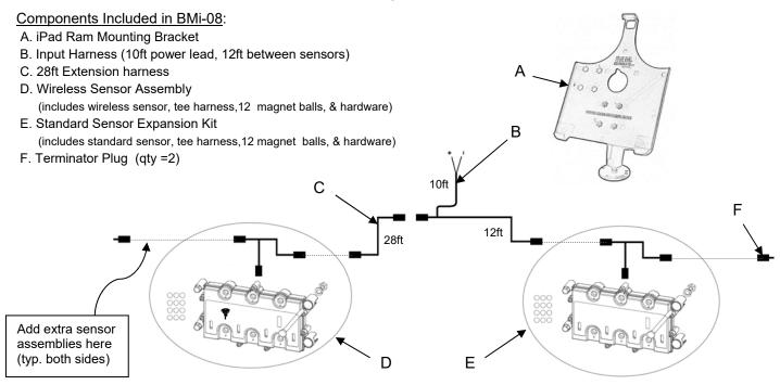
**Step 2:** If the harness lengths supplied are not long enough for your machine measurements, you can order more of these harnesses and add them anywhere in the circuit:
